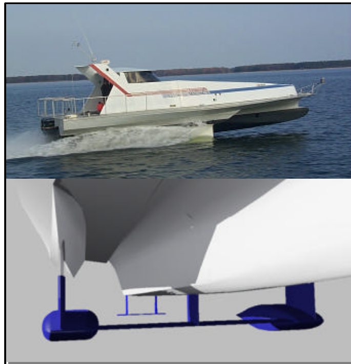
Figure 5 Lifting Body Testing on 7.5 LT Test Craft in Chesapeake Bay
