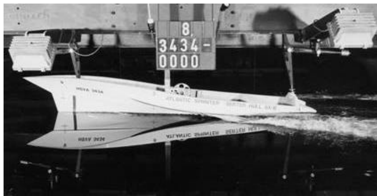
Figure 7 Serter Deep-V Hull Form Model Test
