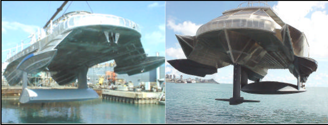
Figure 8 MIDFOIL Lifting Body Technology Demonstrator: Original (left) and Modified (right)
