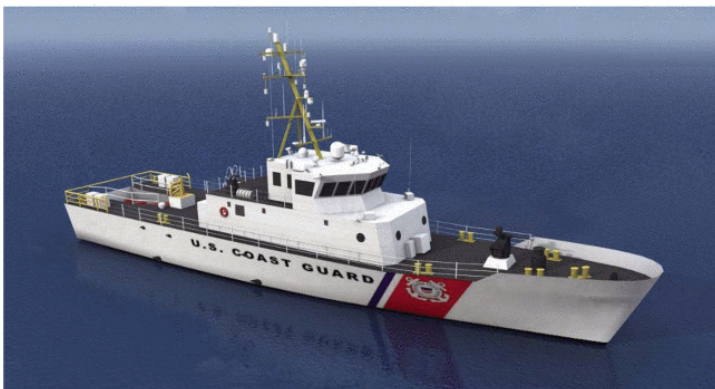
The Fast Response Cutter program was suspended this spring by the Coast Guard because of technical concerns and weight issues with its composite hull design. A new proposal for a 150-foot cutter, the PCX-150, also features a composite hull, but touts the use of lightweight composite panels that have already been produced and approved by the Department of Homeland Security.
