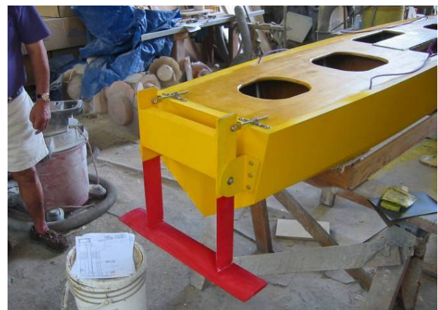
Figure 17 Aft Foil Used in Model Test
