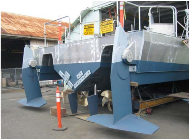
Figure 18 BLB-70 Stern View Showing T-Foils
